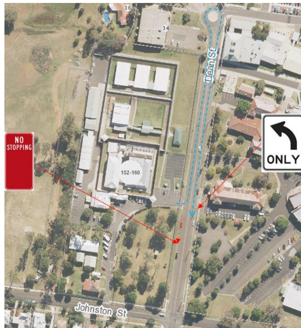
Figure 1: Showing sign placements for Tamworth Correctional Centre exit.
